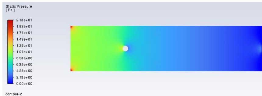
Figure 4b. Static pressure contour at Re = 1 showing a stronger downstream pressure gradient and increasing pressure-drag contribution.
